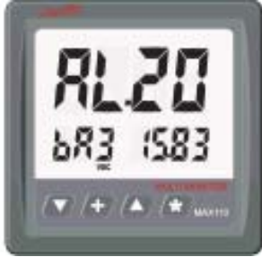
Alarm Source # 20 Battery #3 Volts
