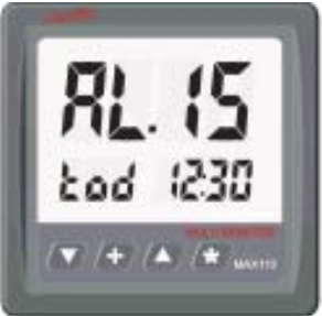
Alarm Source # 15 Time-Of-Day
