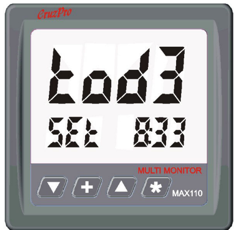
Figure 22 - Clock/Alarm Editor Setting the eight Time-Of-Day Alarms
